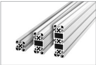
Strut profiles, 10 mm slot, 50 mm modular dimension (p. 2-50)
