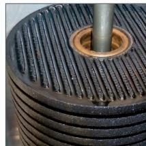
Varnish Removal insert, VRi, after filtration
