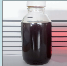
Turbine oil BEFORE filtration with the VRU
