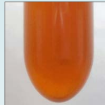
Ultra Centrifuge test, sample after a single pass through the VRU (outlet)
