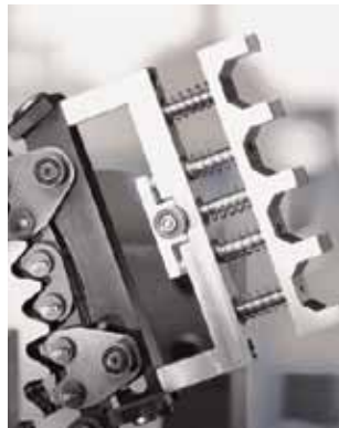
▲ Easy integration of special links as drivers
