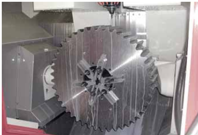
▲ Customer-specific sprocket manufacturing
