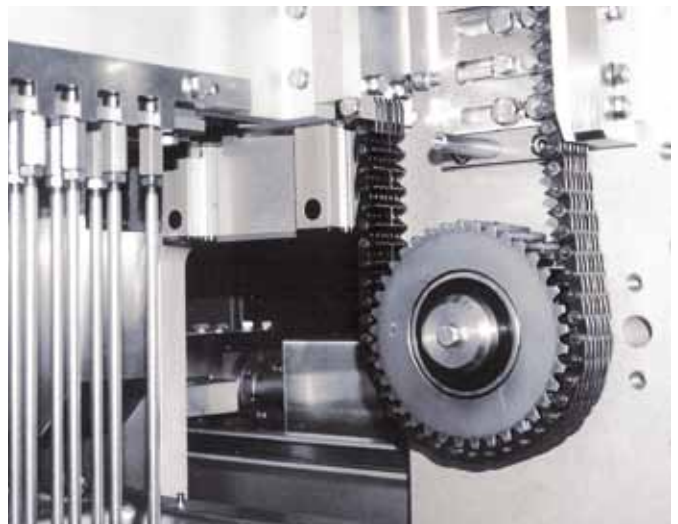
▲ HPC inverted tooth chains in chocolate dosing equipment in the food industry
