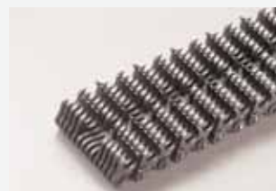
▲ Driver link plates for cross-bars
