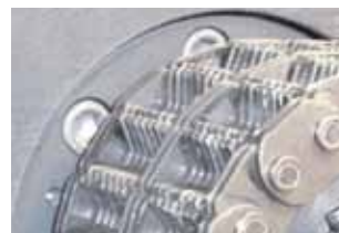
◀ Drive chain with reinforcement plates, combination of center and side guide
